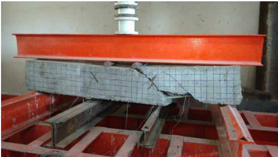
FIGURE 4.31 The crack patterns and ultimate failure of GC.4.2.
