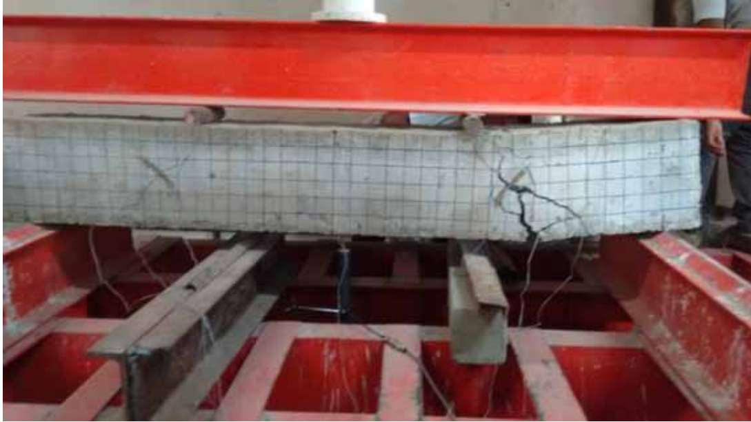
FIGURE 4.4 The crack patterns and ultimate failure of GA.1.1.
