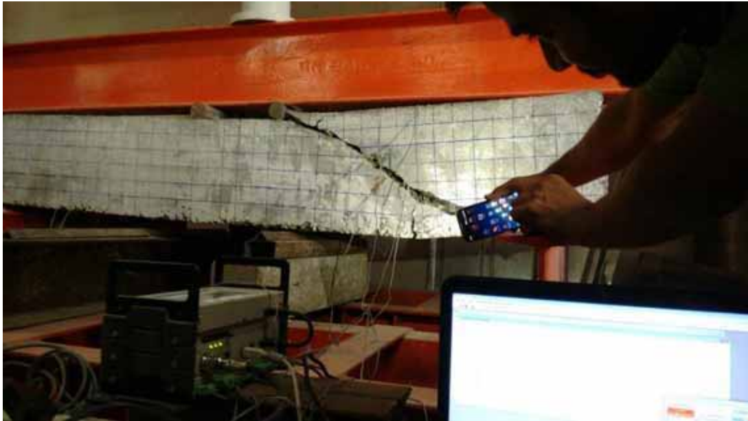
FIGURE 4.28 The crack patterns and ultimate failure of GC.4.1.
