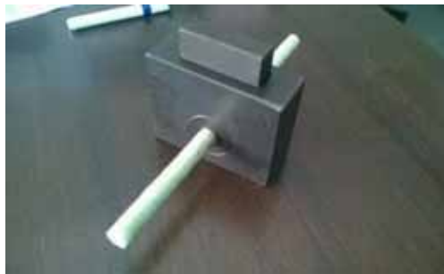
FIGURE3.7 Sample for shear test on GFRP bar
