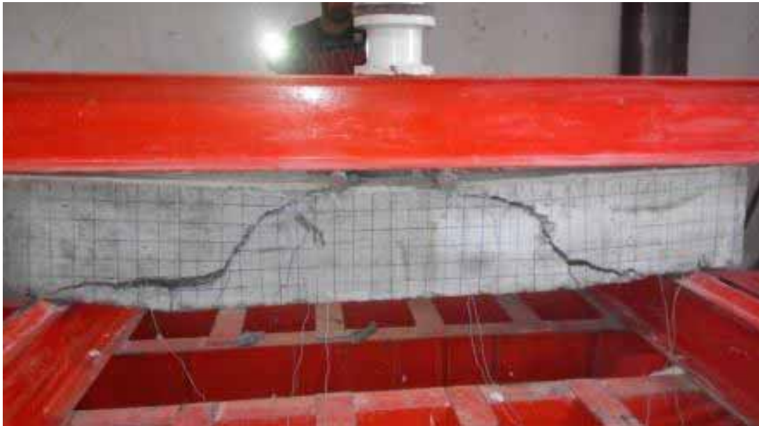
FIGURE 4.34 The crack patterns and ultimate failure of GC.5.1.
