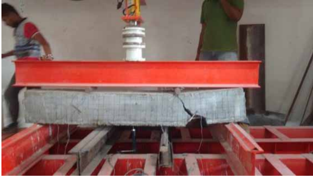
FIGURE 4.13 The crack patterns and ultimate failure of GA.2.2.
