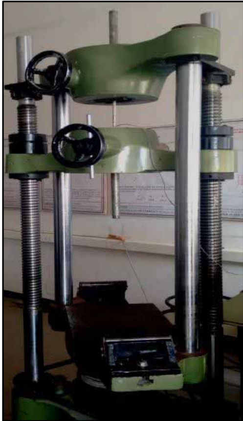
FIGURE3.5 Loaded sample in UTM for tension test of GFRP bar
