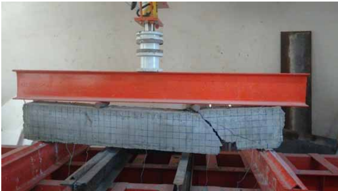
FIGURE 4.10 The crack patterns and ultimate failure of GA.2.1.
