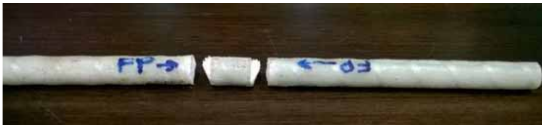
FIGURE3.9 Sample of GFRP bar failed in shear test
