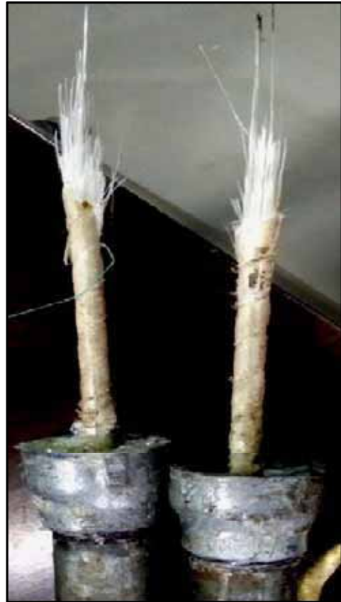
FIGURE3.6 Failed sample of GFRP bar in tension
