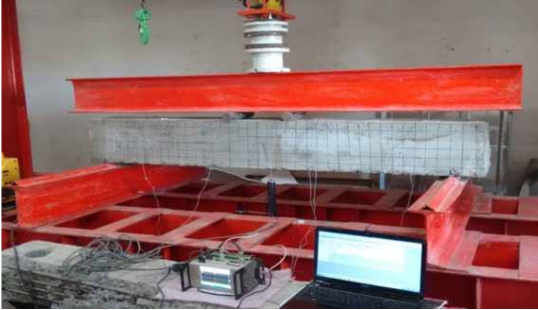
FIGURE 3.28 Gauges & displacement transducer connected to multi recorder TMR-200
