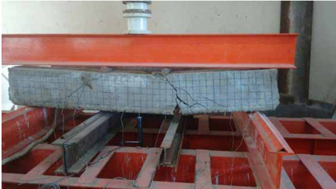
FIGURE 4.19 The crack patterns and ultimate failure of GB.2.2.
