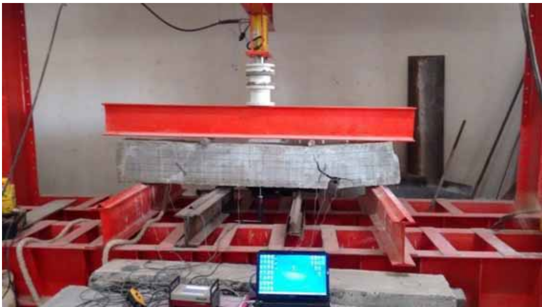
FIGURE 4.7 The crack patterns and ultimate failure of GA.1.2.
