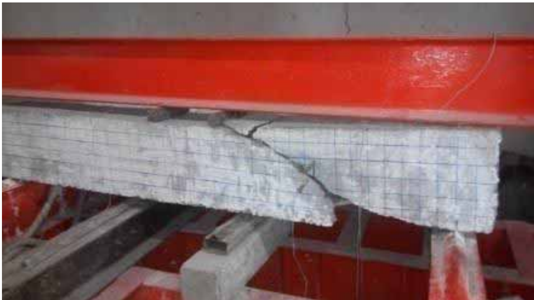
FIGURE 4.16 The crack patterns and ultimate failure of GB.2.1.
