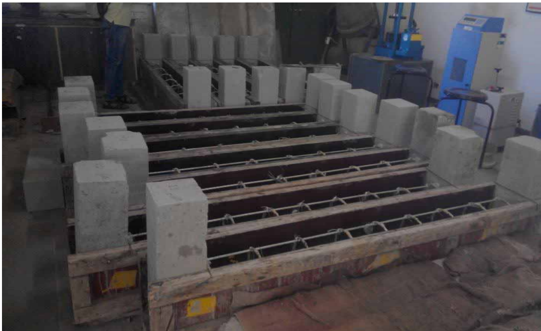
FIGURE 3.24 Bird view of the reinforcement cages placed in the plywood formwork
