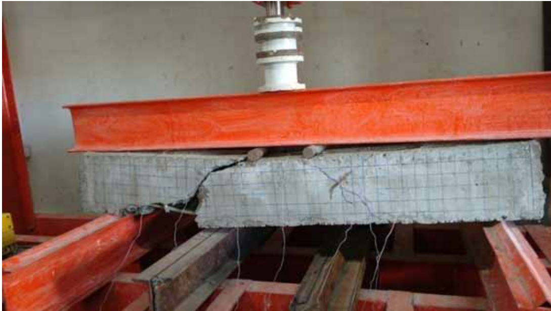
FIGURE 4.37 The crack patterns and ultimate failure of GC.5.2.
