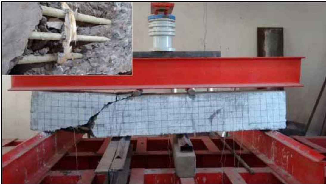
FIGURE 4.25 The crack patterns and ultimate failure of GB.3.2.
