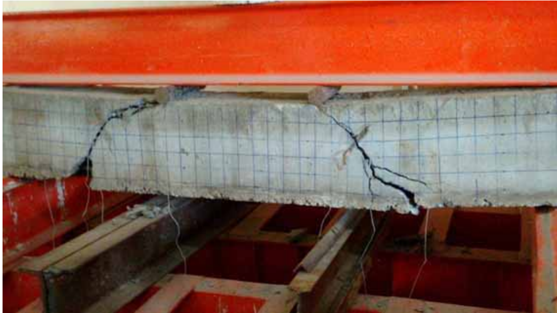
FIGURE 4.22 The crack patterns and ultimate failure of GB.3.1.
