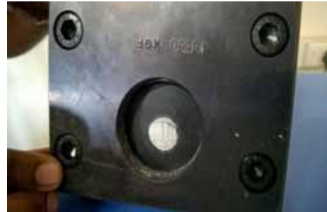
FIGURE3.8 Assembly with failed sample of GFRP bar in shear
